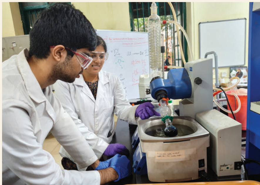
Second-year UG student Divyansh Arora (left) operating a Rotavapor under the supervision of TA Akshata Raveendra Hegde (right). A Rotavapor is used to evaporate volatile organic solvents at much lower temperatures by lowering the pressure in the flask, to isolate pure compounds dissolved in the solvent
