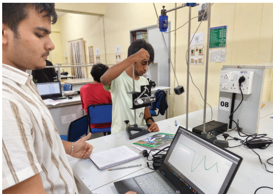
First year UG student Advay Javali (right) launches a ballistic pendulum, whose bob has a rotary motion sensor to track its angular position and velocity. The data is recorded on a laptop operated by Aditya Kumar (left), another first-year UG student. The experiment is meant to verify the conservation of angular momentum
