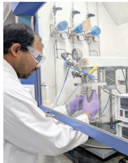
High-pressure reactor unit for direct biomass valorisation to fuels and chemicals at severe reaction conditions
