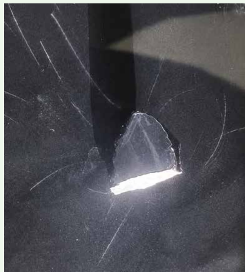
Long, cloudy tracks of otherwise invisible particles can be seen with the help of the monazite
