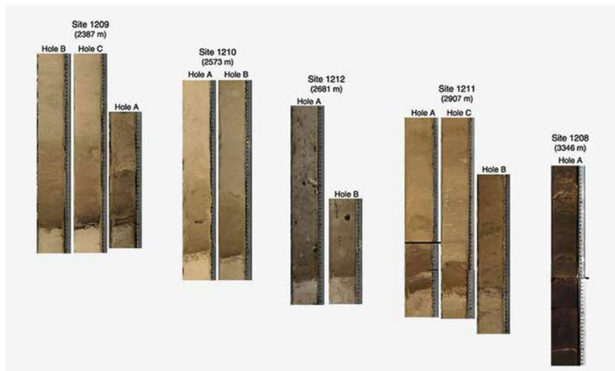
Sediment cores from Shatsky Rise, an underwater volcanic plateau in the northwest Pacific Ocean, ordered by depth. The transition from carbonate (white) to clay (brown) reflect the abrupt ocean warming during the Palaeocene–Eocene Thermal Maximum
