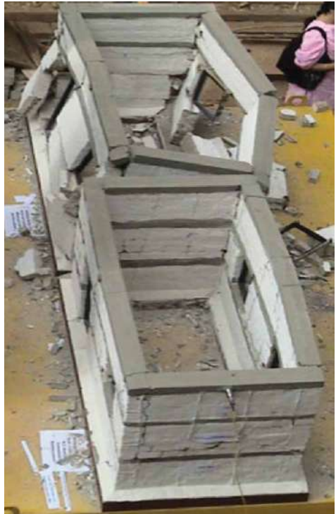
Behaviour of masonry building models with and without near surface containment reinforcement, subjected to horizontal base motion on the shock table
