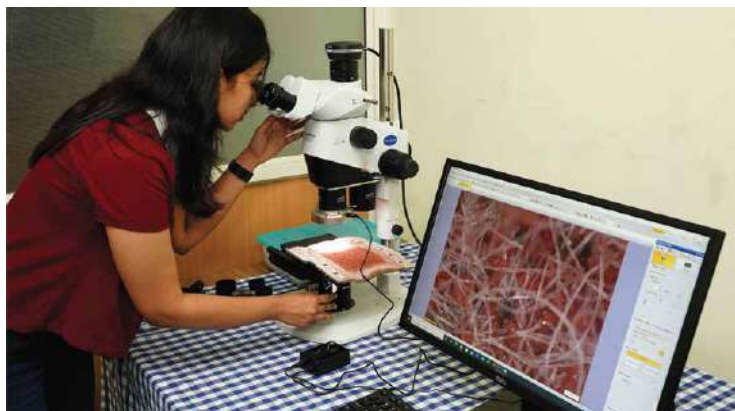
Anjali Pillai, a PhD student in Madhavi Latha's lab, using an optical microscope to study the interaction between geosynthetic clay liner and M-sand particles
