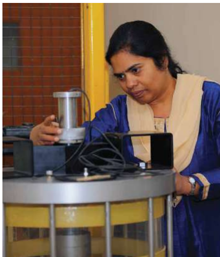
Madhavi adjusting the loading plunger in a large diameter cyclic triaxial test setup – used to check for soil liquefaction
