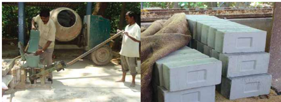
Fluoride contaminated sludge being converted (left) into safe building brick (right)
