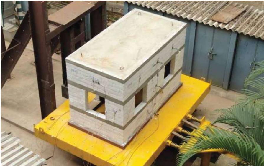
KS Nanjunda Rao built a large shock table to test earthquake resistance of buildings
