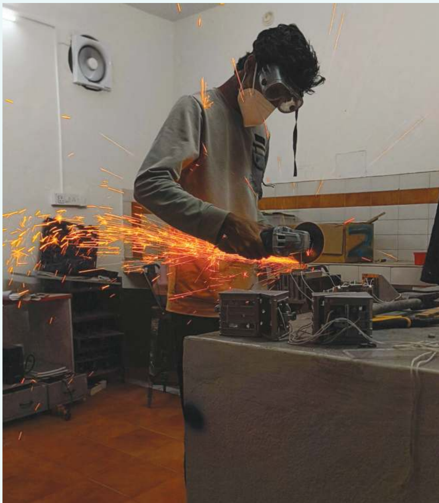
Yash cutting aluminium brackets for making a support channel prototype for his biophilic curtain wall project at the Prototyping Lab, DM, IISc
