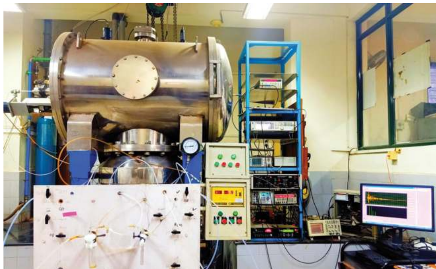
Pulsed nozzle Fourier transform microwave spectrometer built at IPC and used to study the hydrogen bond
