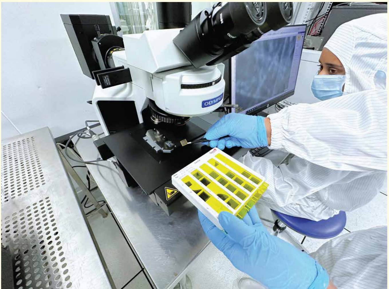
GaN device samples being loaded onto a microscope at GEECI
