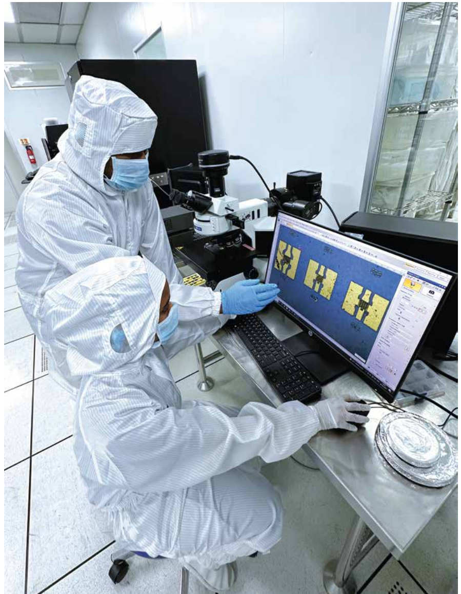
GaN devices being inspected using optical microscopy at GEECI
