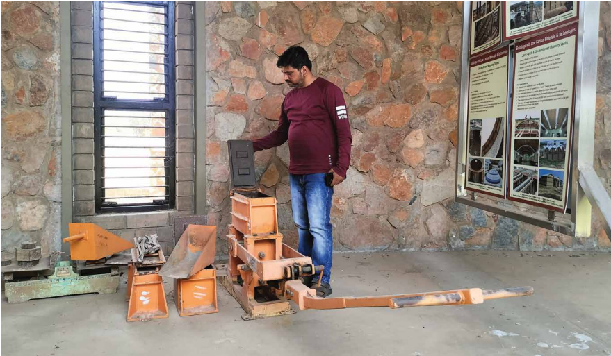
Machine for making Compressed Earth Blocks (CEB)
