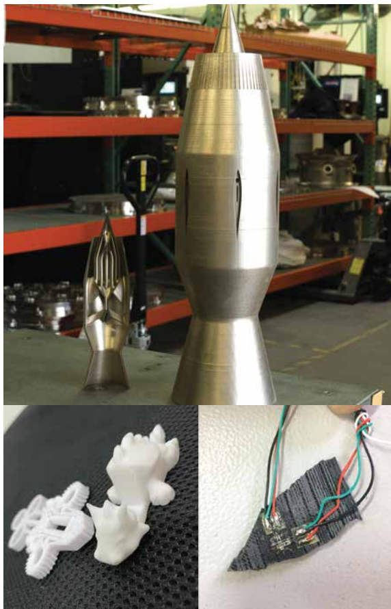
Top: 3D-printed engine made of Inconel 718 alloy; Bottom left: 3D-printed plastic parts; Bottom right: 3D-printed auxetic composite being tested
