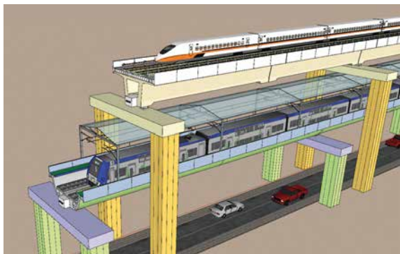
Representative diagram of an innovative three-layer transportation solution given to the authorities to overcome space complication in the city
