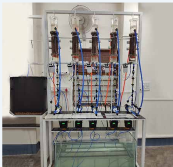
Experimental setup containing a series of fixed-bed biofilm reactors
