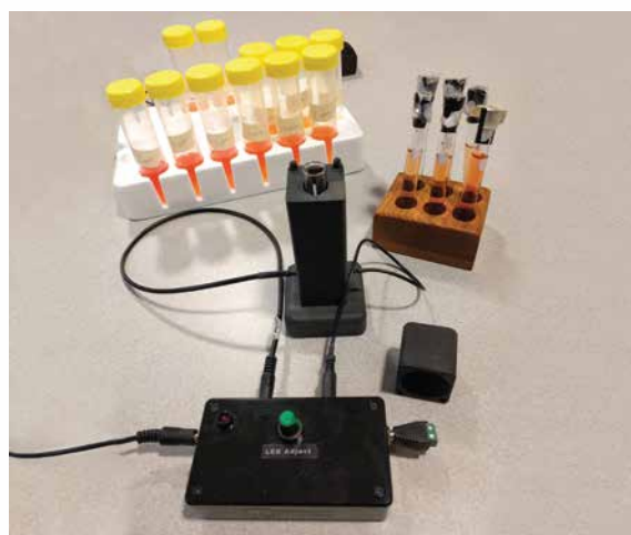
The LED-based spectrophotometer to detect the levels of fluoride, manganese, and iron in water
