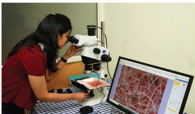
Anjali Pillai, a PhD student in Madhavi Latha's lab, using an optical microscope to study the interaction between geosynthetic clay liner and M-sand particles
