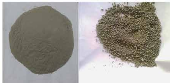
Fly ash (left), a by-product of coal-fired power stations, can be converted to geopolymer sand (right) to use in construction
