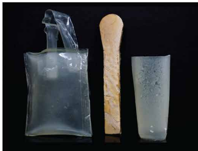
Biodegradable carry bag, cutlery and tumbler made using non-edible oil and cellulose
