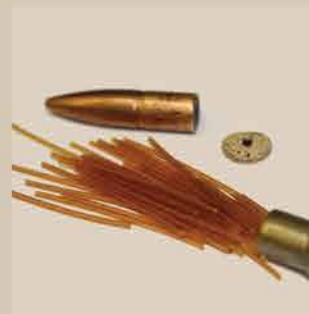
Cordite filaments in a .303 British Rifle cartridge
