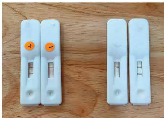
Antigen-based rapid diagnostic kits fabricated in Tatu's lab for trypanosomiasis (left) and trichomoniasis (right). Two coloured lines in the assay indicate the presence of infection
