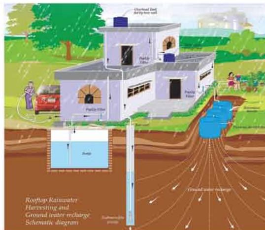
A schematic presenting various levels of rooftop rainwater harvesting and groundwater recharging
