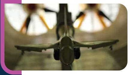
The open-circuit wind tunnel in the old Aerospace Engineering building
