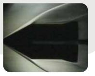
Shockwaves formed in front of a model at high speeds
