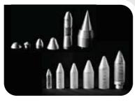
Top row-Satellite launch vehicle (SLV) models tested in shock tunnels; Bottom row-Hypersonic vehicle models with different forebody shapes tested in shock tunnels
