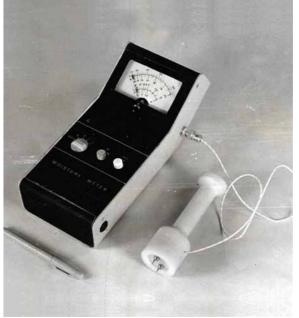
An electronic moisture meter developed as part of an early project at CEDT
