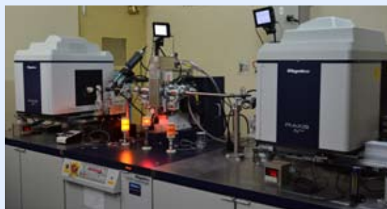
An X-ray generator with an imaging plate recording the intensity of diffracted rays
