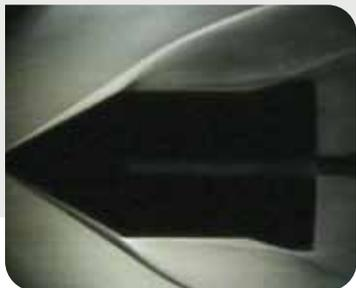
*Shockwaves formed in front of a model at high speeds*
