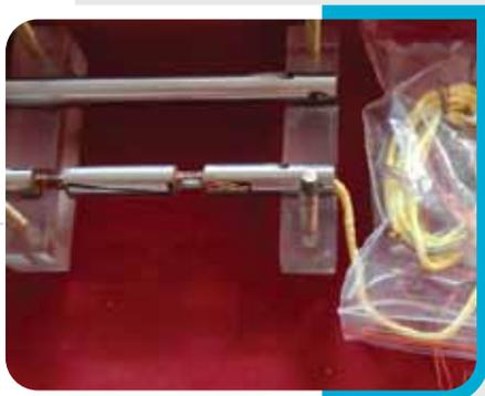
*A strain gauge balance*
