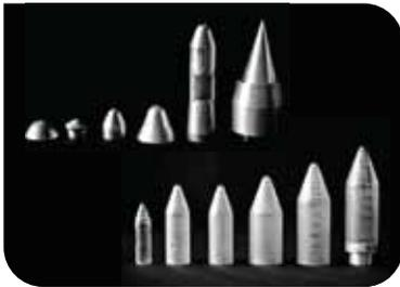
Top row: Satellite launch vehicle (SLV) models tested in shock tunnels; Bottom row: Hypersonic vehicle models with different forebody shapes tested in shock tunnels
