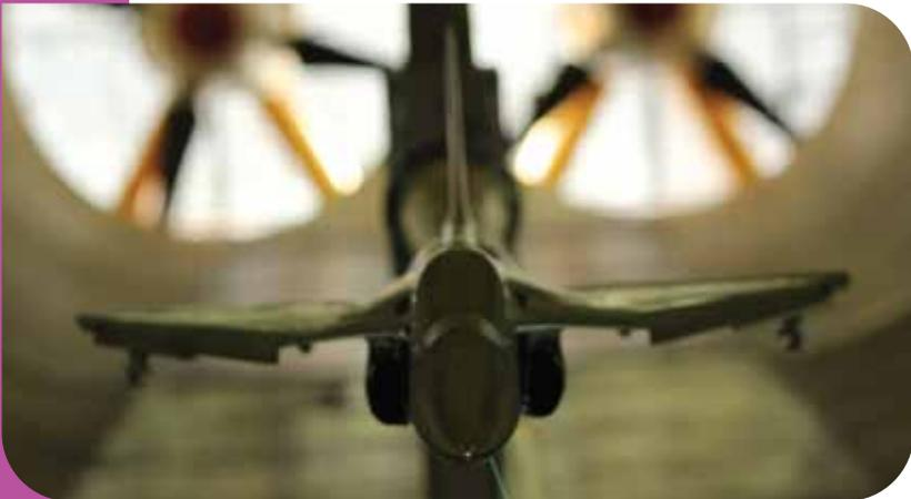
*The open-circuit wind tunnel in the old Aerospace Engineering building*
