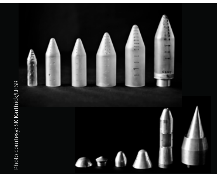
Top row: Satellite launch vehicle (SLV) models tested in shock tunnels; Bottom row: Hypersonic vehicle models with different forebody shapes tested in shock tunnels
