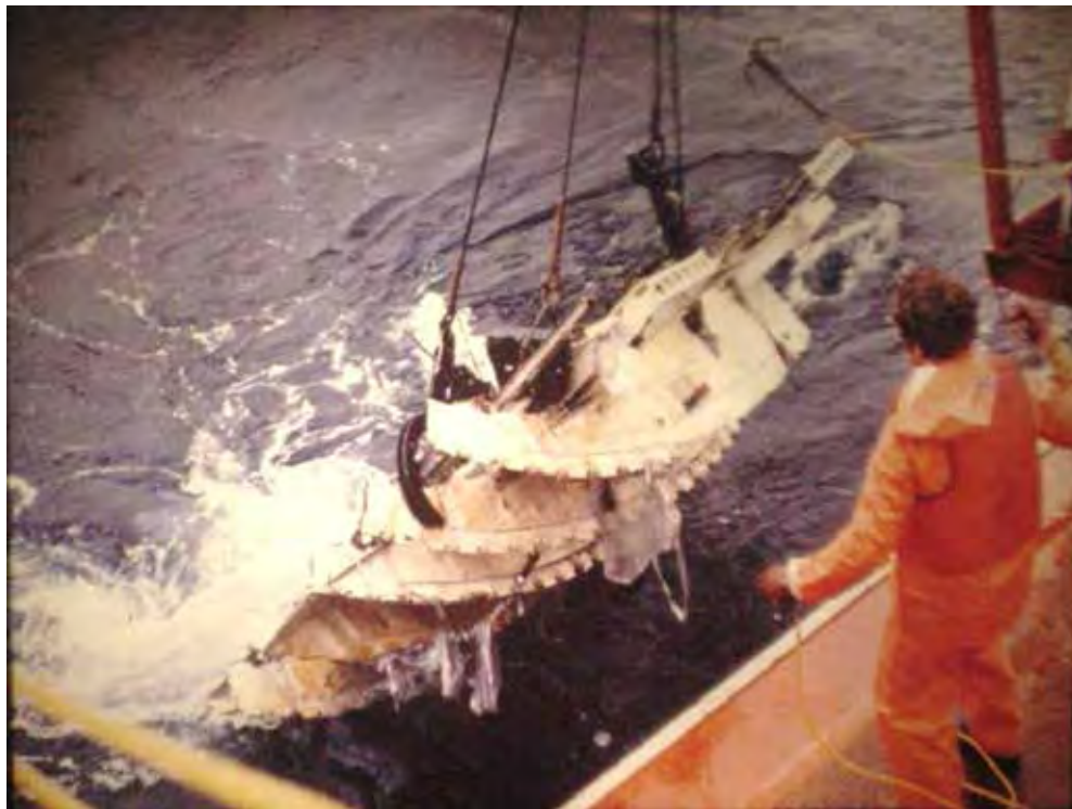
A part of the floor structure of Kanishka being recovered from the ocean floor (Photo courtesy: V Ramachandran)
