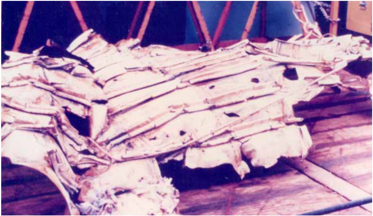
Bottom skin of the front cargo hold showed evidence of explosive deformation and fracture (Photo courtesy: V Ramachandran)
