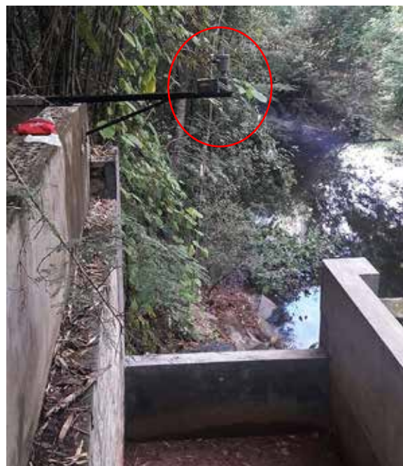
A water-level sensor indicated by the red circle was installed as part of a pilot project in the IISc campus
